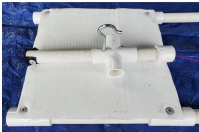
Made from a PPR 20 tube, a tee and a plug. For ease of gripping, a hook is installed in the tee. A 4 m long rope is attached to the plug (the length can be shortened). The other end of the rope is tied to the docking station. Velcro tape (hooks) is attached to the end of the connector. The connector is weighted and is initially located on the docking station platform.
