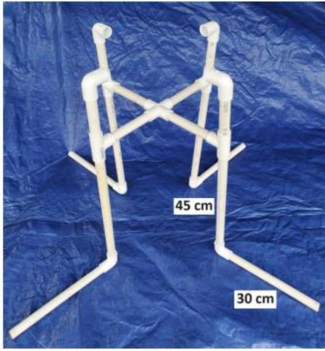
Made from pipes ppr 20 and fittings of the appropriate size. The lower part of the structure is weighted.
