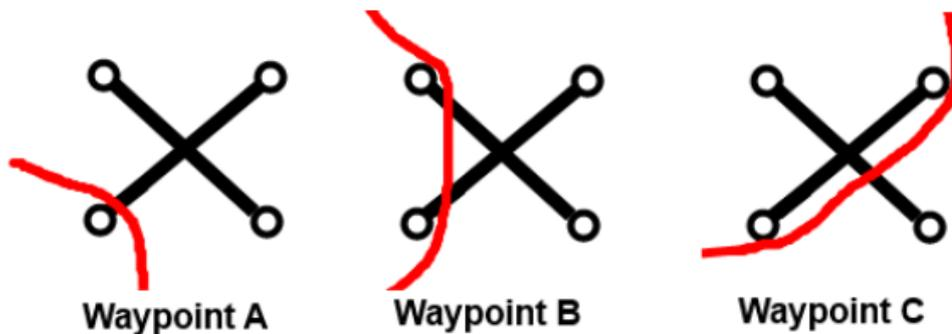
*Waypoint A is an unsuccessful cable lay, as the cable is inside one vertical post only. Waypoint B is a successful cable lay, as the cable is inside two vertical posts. Waypoint C is an unsuccessful cable lay, as the cable is only inside one vertical post (the lower right post only).*
