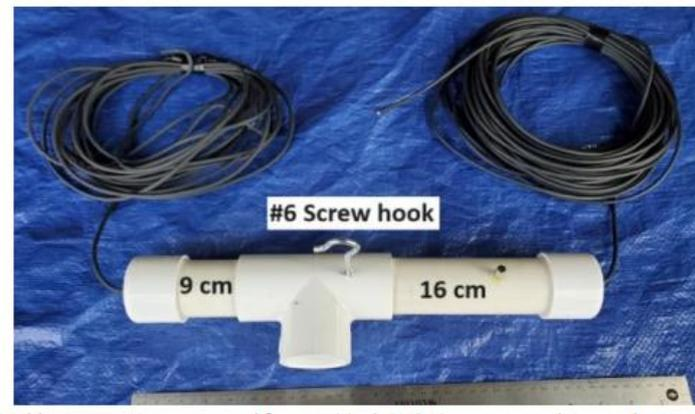
Made from pipes ppr 50, two plugs and a tee of the appropriate size. A hook is provided for gripping. A cable is attached to both sides of the repeater. The
